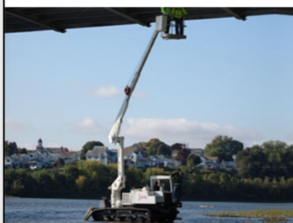
Fig. 1 A land based bridge truck that operates in water depths up to 9ft.
